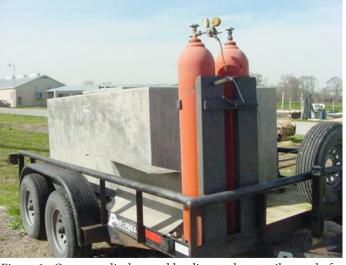
Figure 1. Oxygen cylinders and hauling tank on trailer ready for transport. Photo: Greg Lutz
