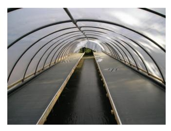
At the end of the raceway, a plastic stock tank (a tank for watering livestock) is positioned under the edge of the liner hanging off the raceway. A 2x4 is placed on its side under the liner to create a small dam that will set the water level in the raceway. A simple piece of window screen laid across the end of the raceway will reduce plant material from getting into the tank.
