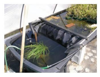
A circulation pump is placed in the tank and tied into a 1/2" irrigation pipe that is tacked onto the side of the raceway leading back to the far end of the raceway. The water is lifted, carried to the top of the raceway, and then dropped to recirculate past the plants back to the tank where it is again pumped around again. A pump with 90 gallons per hour would be fine.
