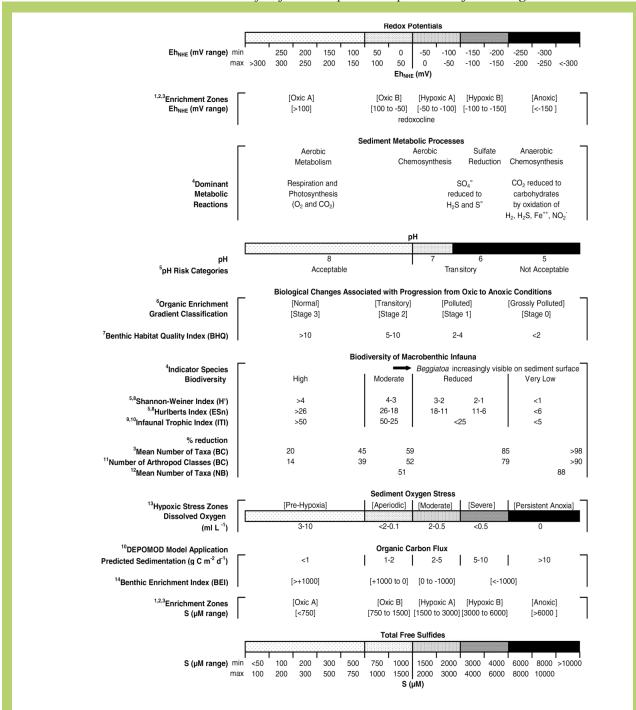
**Figure 3.** Nomogram depicting relationships between common geochemical and biological indicators of marine sediment condition below marine fish farms. Copied with permission from Hargrave et al. 2008.
