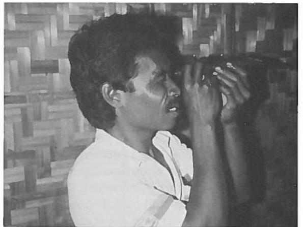
Photo 43. Salinity readings are taken routinely once a week unless during the rainy season (then refractometer readings may be required more often).
