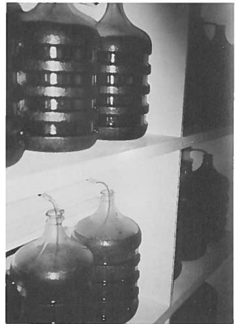
Photo 24. Algae production in 19-liter, or 5-gallon, clear plastic bottles (these are safer to handle and transport than the glass but are more difficult to clean).
