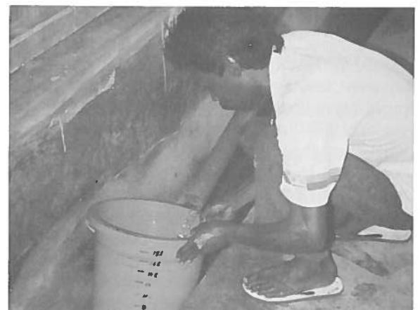
Photo 41. Effluent flow rate is checked daily at the maturation tank to maintain a constant, stable environment.
