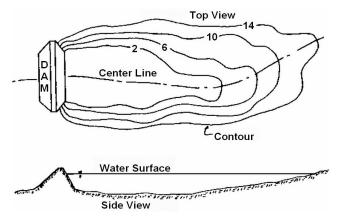
Excavated ponds are constructed by excavating a pit below the normal ground level. These ponds work well in areas which have naturally high water tables. These types of ponds generally require more earth to be moved than embankment ponds for comparable storage. Therefore they are generally used when embankment ponds will not work. (Figure 2)
