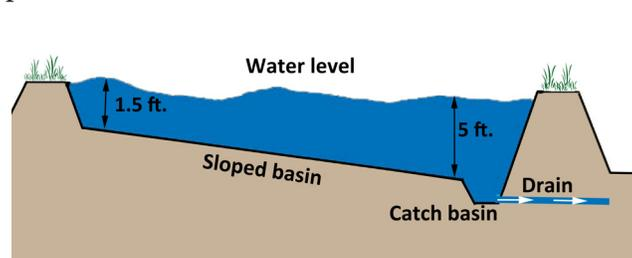
Figure 2. Lateral diagram of ideal pond form.
