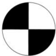
For the purpose of estimating algal density in a pond, a modified and simplified application of the same principle is appropriate. Because our use of the disk is simply to estimate the relative density of an algal bloom as being either too heavy or too light one can eliminate the concept of establishing an SDA and use a less sophisticated approach.
