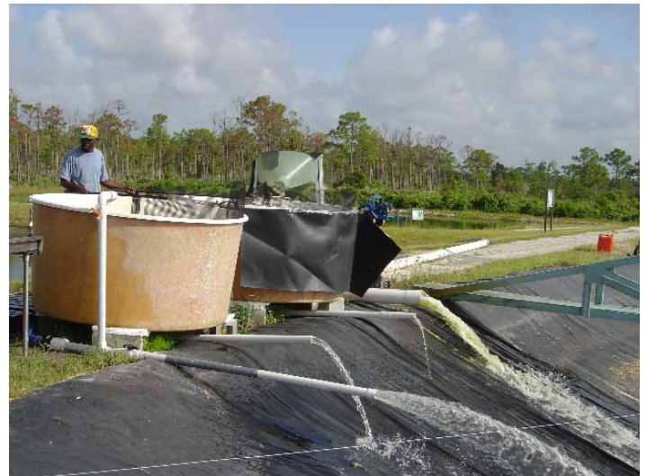
Figure 3. The arrangement of the green dewatering tower and the two round holding tanks on the levee.
