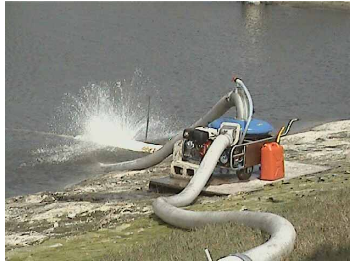
Figure 2. Fish pump operating from the outer-bank of the retention pond.
