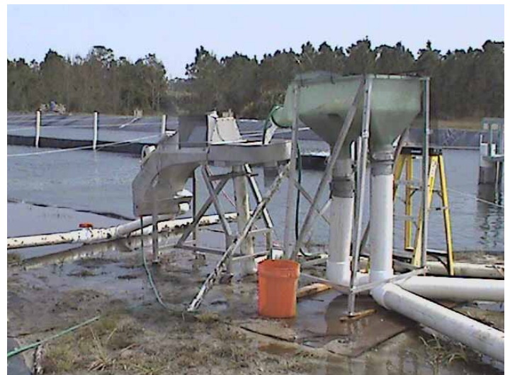
Figure 5. Incorporation of the shrimp counter (left) with the dewatering tower. Credits: Scott W. Grabe
