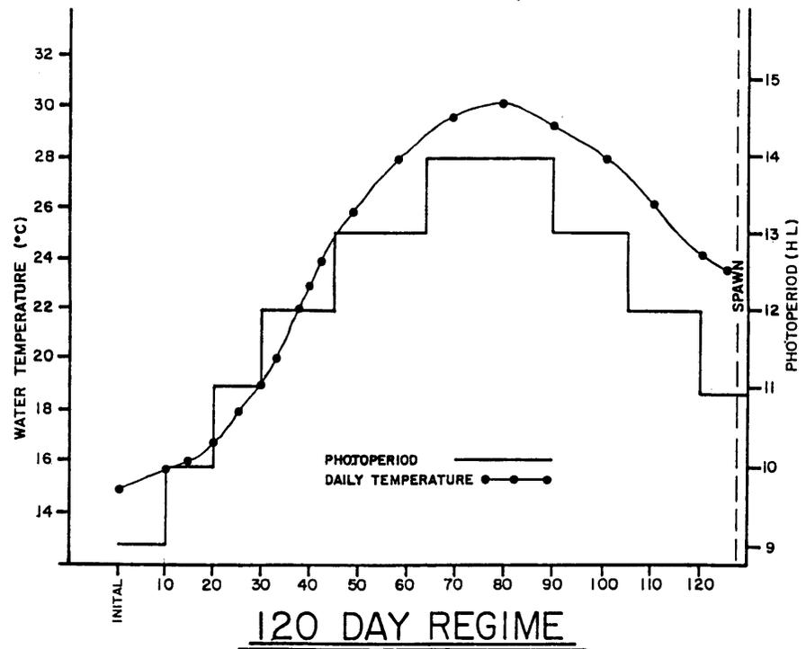
Figure 1. A 120-day induced maturation cycle is imposed under controlled photothermal conditions.
