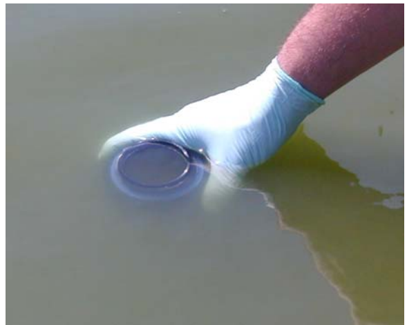
Figure 3. Seal under water to avoid trapping air
