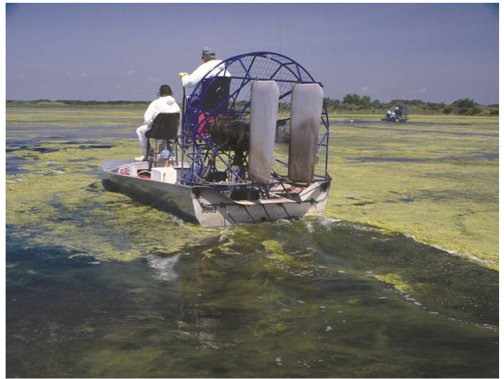
Figure 6. An application of aquatic herbicide using an airboat with trailing hoses for treating hydrilla. Note: Filamentous algae is on the water's surface and hydrilla is below.
