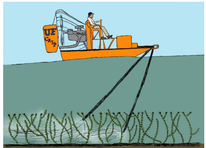
Figure 1. Bottom acre-foot treatment with weighted trailing hoses. This system delivers the herbicide directly into the weed bed for maximum efficiency and lower cost. Credits: Line illustration drawn by Lyn Gettys and colored by Josh Huey.
