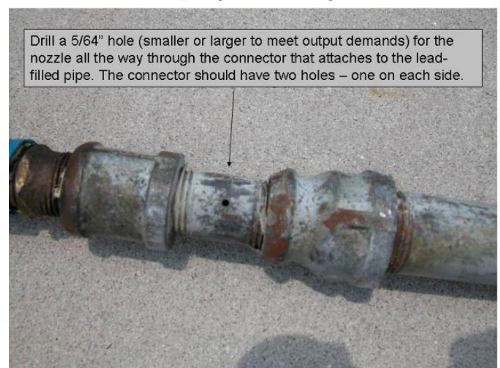
Figure 3. The nozzle for herbicide discharge can be drilled to any appropriate size. Note that the leading edges of the fitting are ground down to minimize snagging on submersed weeds.
